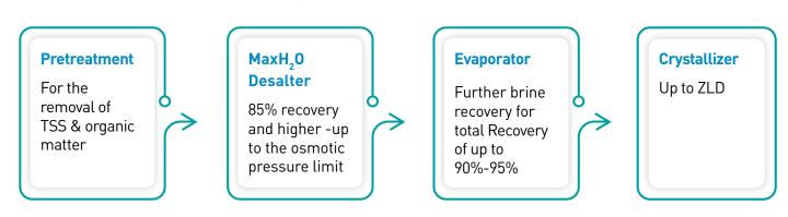
Efficient waste management and disposal is the cornerstone of sustainable development. With increasingly stringent regulations on sea, river, and deep well injection, the implementation of advanced water treatments is critical. Treatment of cooling tower effluents usually requires the use of several technologies to meet the required discharge level - up to ZLD. These can inclue filtration to membrane treatment, followed by thermal technologies such as evaporators and crystallizers.
